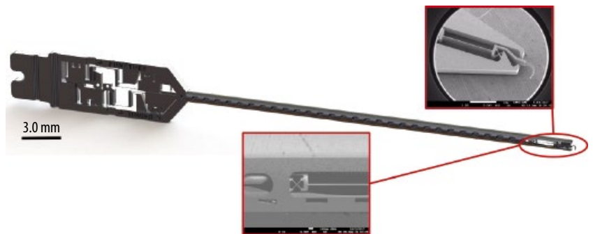
Fig. 1 Safe puncture tool made of a single glass substrate (Source: Instant Lab & Galatea Lab)
