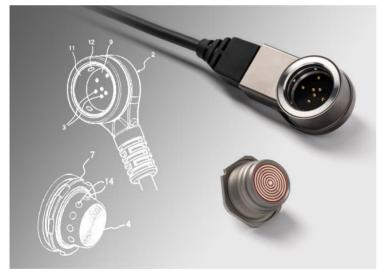
**Fischer LP360<sup>™</sup> 7-pin connector receptacle and plug**: up to 3x 5A power and 4x 1A signal contacts. Contacts on the receptacles are concentric "tracks", those on the plug are pins. Locking is performed thanks to special ogive-shaped elements positioned on the inner diameter of the plug body. (Illustration on the left: drawing from the patent)
